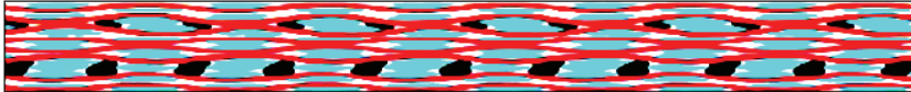
Figure 14. Whole composite structure (Tomkova, 2006) (blue – crosswise fibre bundles, red – lengthwise fibre bundles, black – voids, white – matrix)
