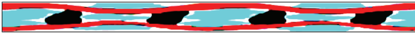
Figure 13. Structural model of Lamina (Tomkova, 2006) (blue – crosswise fibre bundles, red – lengthwise fibre bundles, black – voids, white – matrix)
